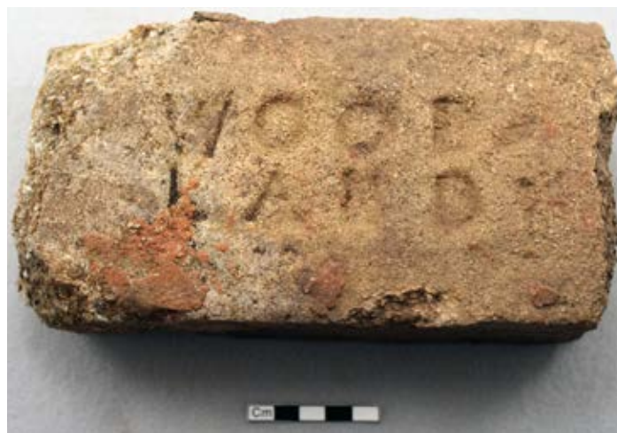
Firebrick discarded during routine blast furnace relining at Catoctin Iron Furnace, Frederick County. This brick was manufactured by Woodland Fire Brick Co, Clearfield Co., Pennsylvania. Image courtesy of Elizabeth A. Comer.
