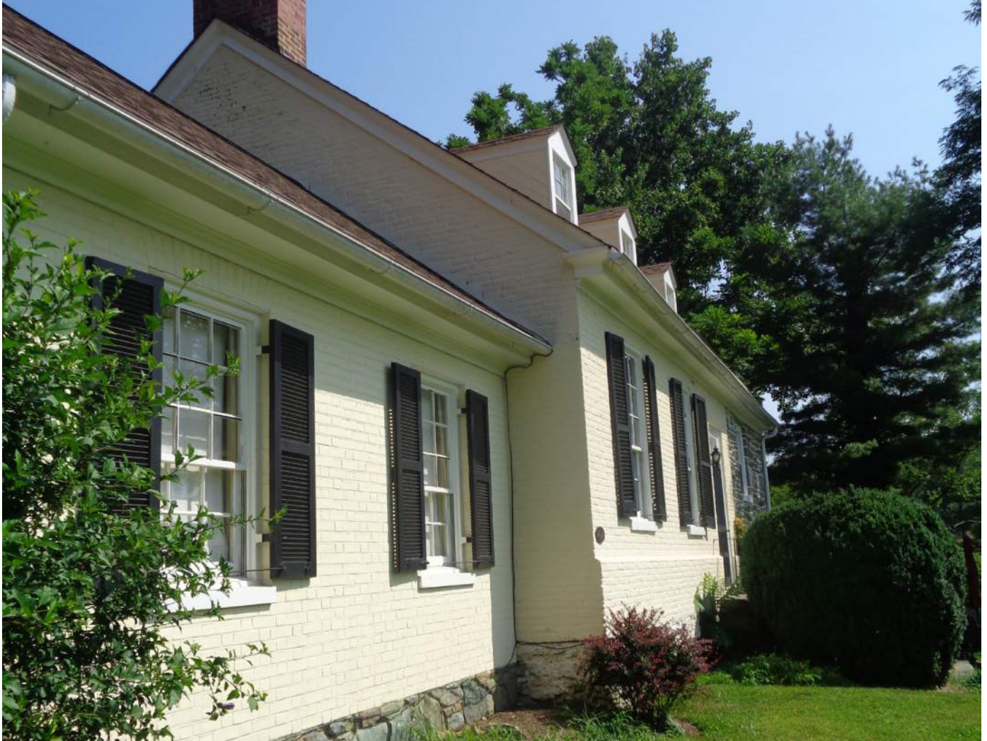
The 1960s brick addition (left) at Still Work is recessed from the original one-and-a-half story section, but the materials and detailing are in keeping with the original. Photo by authors.
