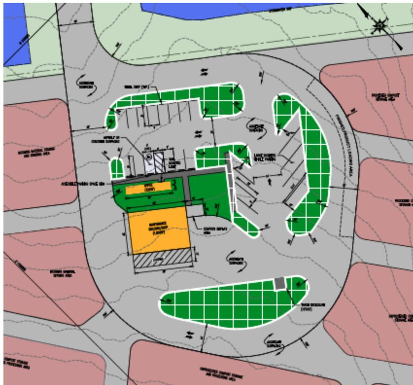
The turning radii for the driveway and circulation around the office and parking lot are maximized to serve a semi-truck, the largest and most infrequent truck size for the Property. **Exhibit I.**
