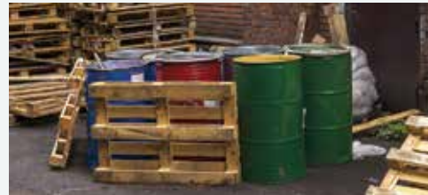
Not Using Secondary Containment
