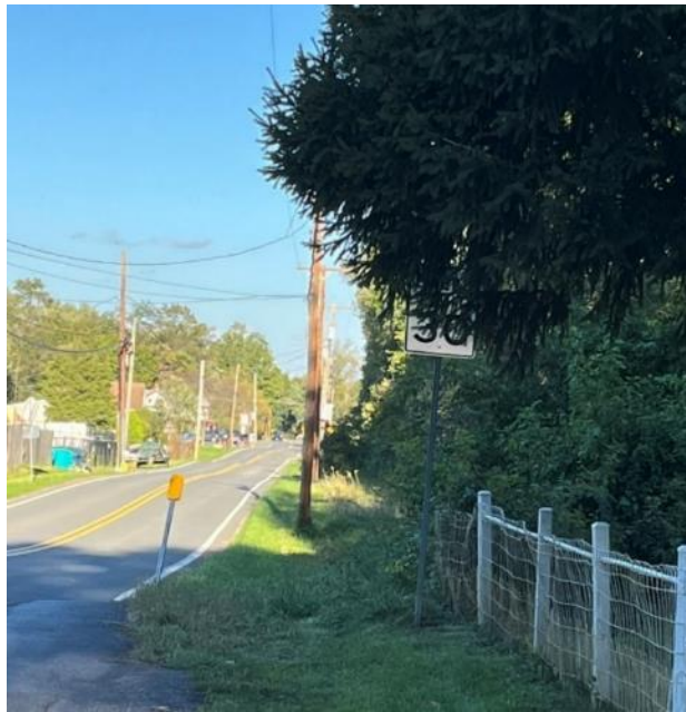
Figure 22: Poorly visible speed limit sign near Mountaindale Road at Bethel Road Intersection.
