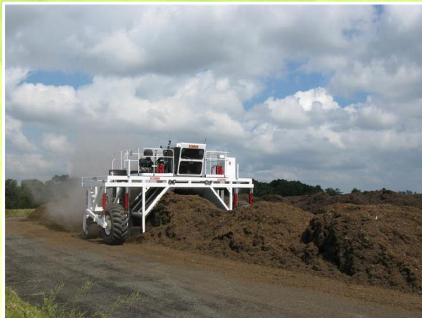
Compost windrow being turned at the Reichs Ford Road facilities.
